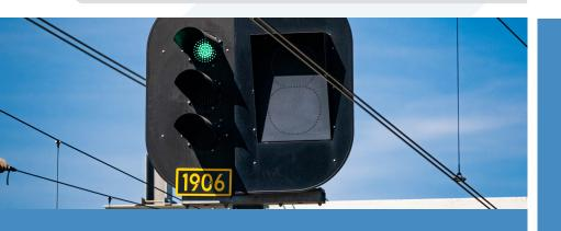
The lenses are in the form of numbers, letters or symbols for the purpose of conveying information to the driver. An MSG2w can display up to 4 different characters in one housing.
